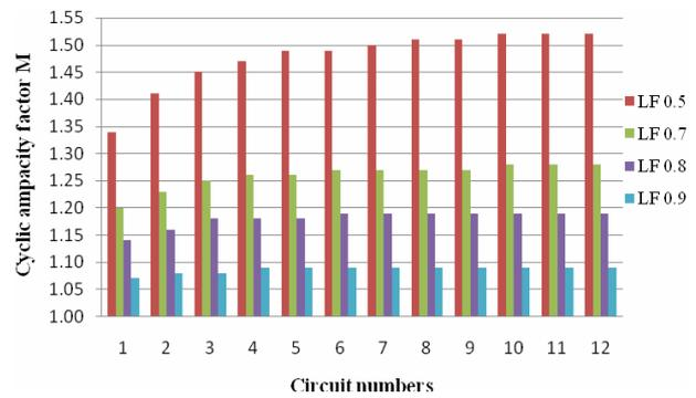
**Figure 3. Relationship between cyclic ampacity factor M and circuit numbers.**
