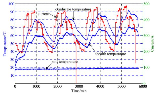
Figure 2. Graph of LF 0.7 single-loop direct buried cable cyclic ampacity experiment.
