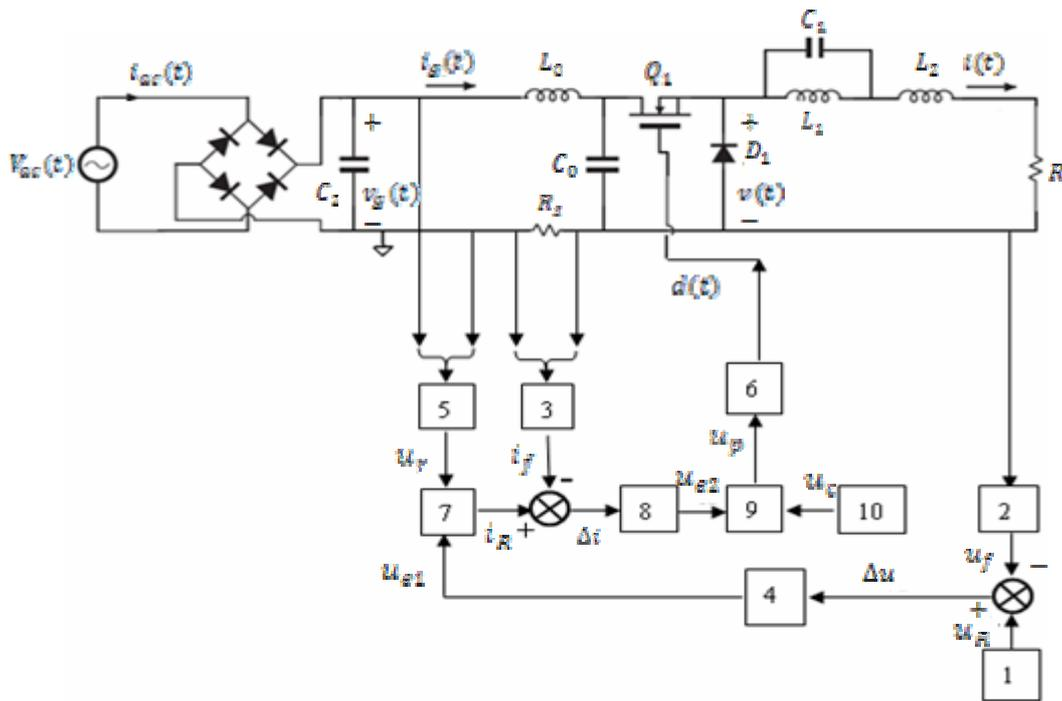
**Figure 5.** Block diagram of the control scheme-double loop: 1- DC voltage reference; 2- DC output current sensing; 3- AC input current sensing; 4- voltage regulator; 5- input voltage sensing; 6- drive circuit; 7- multiplier; 8- current regulator; 9- PWM comparator; 10- sawtooth wave generator.
