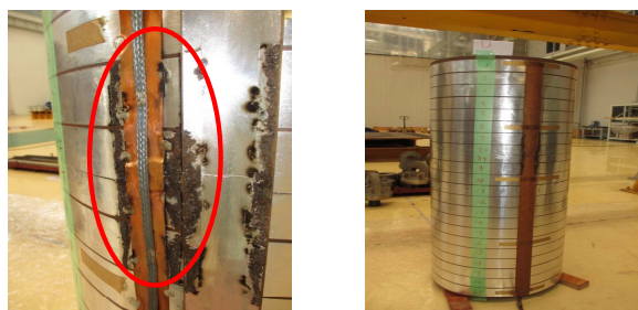
Figure 3. Photo of discharge trace of magnet shield layer.
