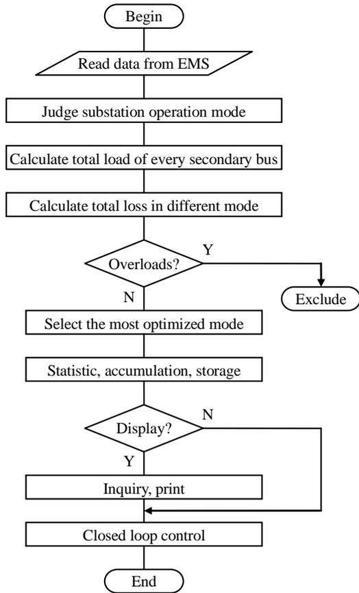
Figure 2. Flowchart of optimization software for substation operation mode.
