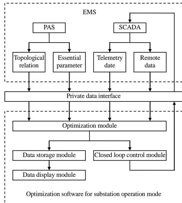
**Figure 1. Framework of optimization software for substation operation mode.**
