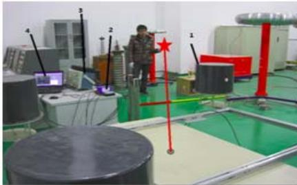
**Figure 5. Testing scene. (1-antenna array; 2-amplifier & filter module; 3-high-speed oscilloscope; 4-laptop).**
