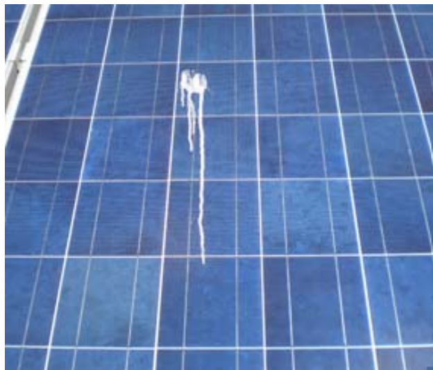
Figure 4. Guano shadows on the PV module.
