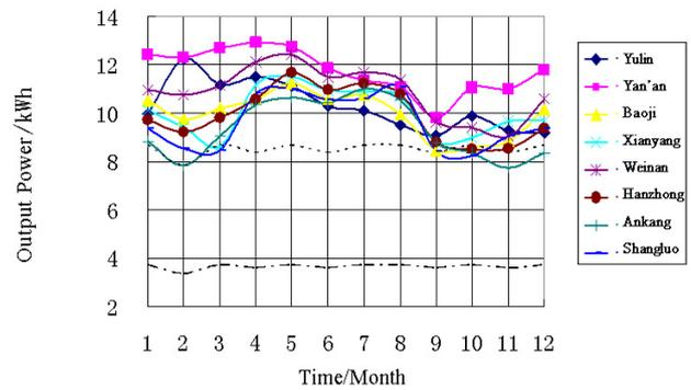
**Figure 6. Output power prediction of off-grid home photovoltaic power system.**
