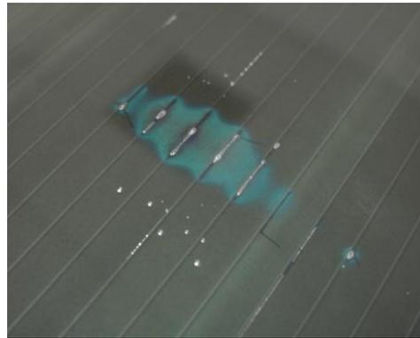
**Figure 7.** Corrosion effect caused on sample 1 module (near central cell of module).
