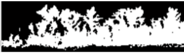
Figure 9. Experimental frosting binary image on the cryogenic surface of finned-tube vaporizer.
