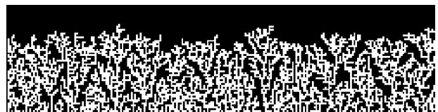
Figure 3. Frosting simulated image on the cryogenic surface of finned-tube vaporizer.
