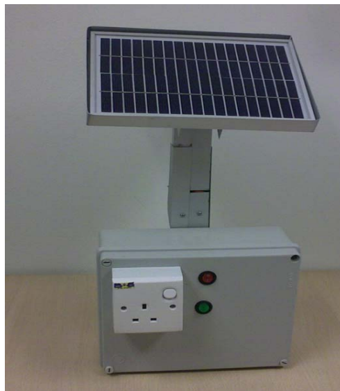
Figure 5. Low Power Solar PV system for low power home electrical appliances.
