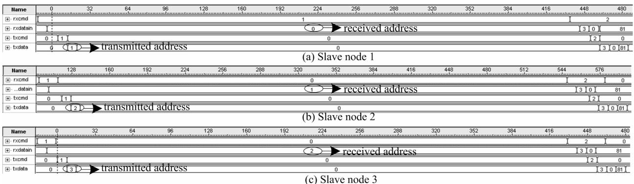
Figure 5. The communication data of delay automatically measured from the slave nodes (1~3).
