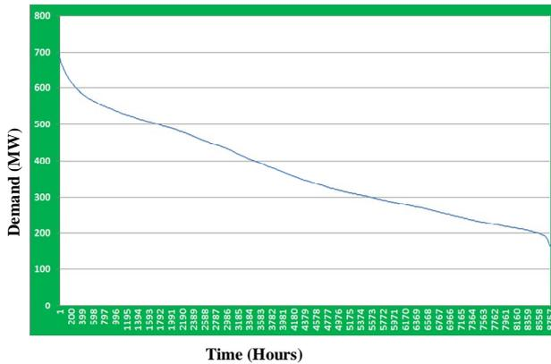
Figure 5. Hail load duration curve.
