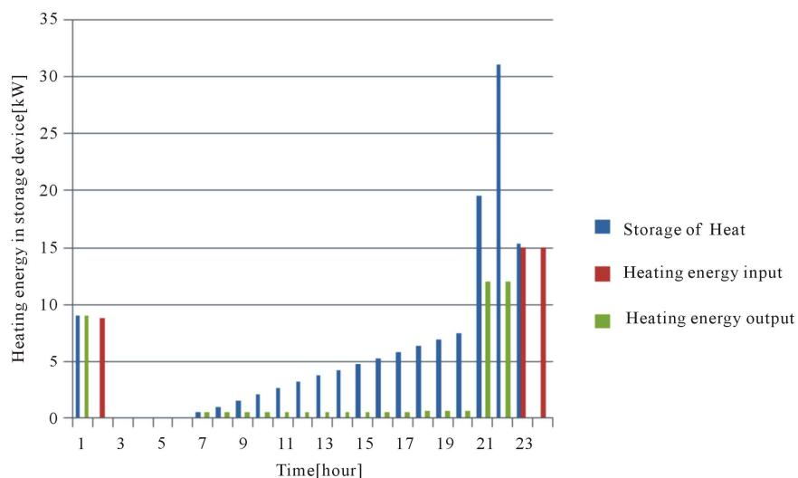
Figure 11. Input, output and storage of heating energy in storage device.
