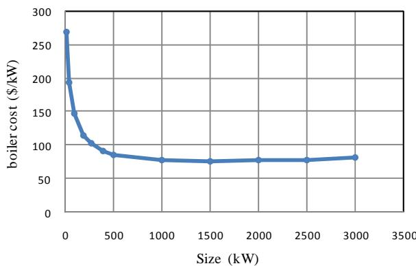
**Figure 8. Boiler cost.****Table 1. Performance characteristics of CHP and auxiliary boiler.**
