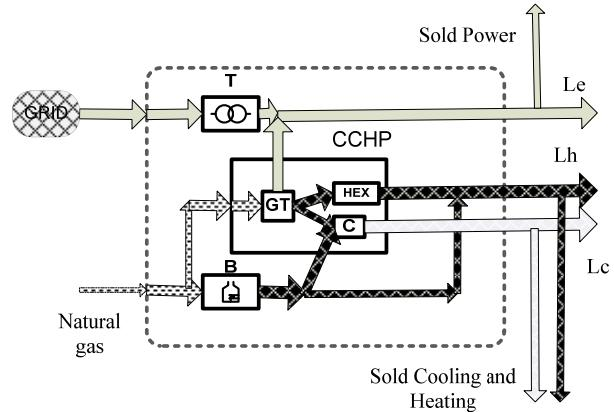
**Figure 1.** An energy hub containing an electric transformer, a CCHP, a boiler (B) an absorption chiller (C): and Heat Exchanger (HEX).
