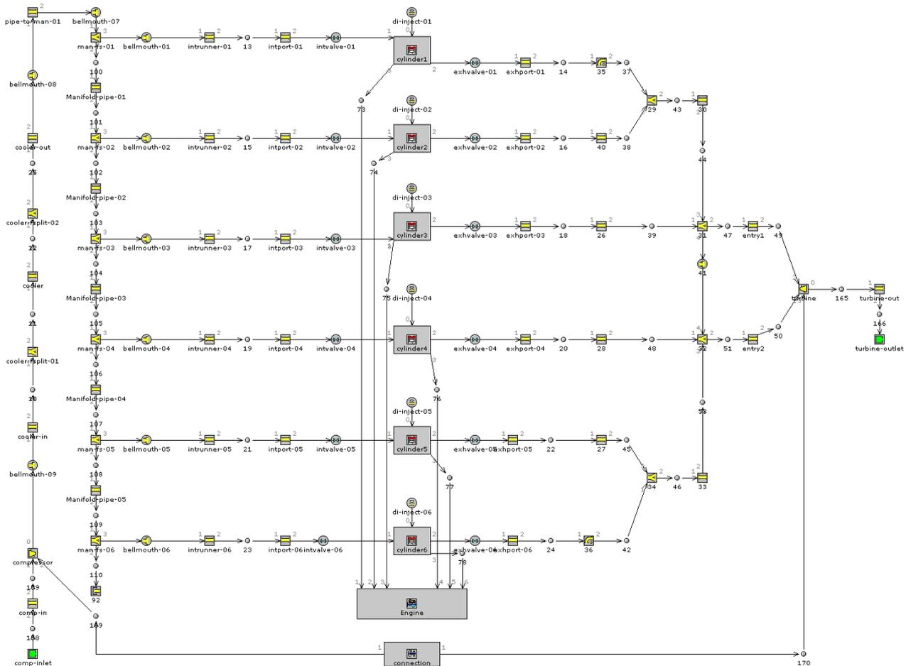
**Figure 1. Diesel engine simulation model diagram.**
