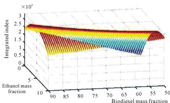
**Figure 3.** Relation between Integrated optimization index (option two) on all kinds of conditions and the proportion of ethanol and biodiesel.
