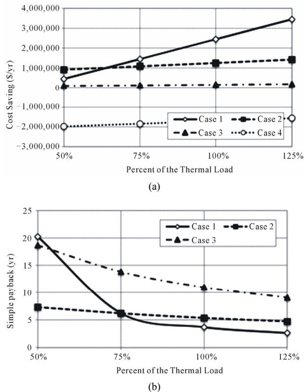
Figure 3. Effect of the facility thermal load on (a) the annual cost savings (b) the simple payback.
