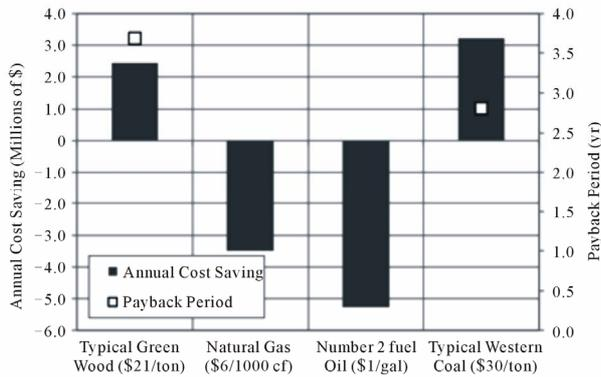
**Figure 4. Effect of the CHP fuel used on the cost savings and payback period for the facility analyzed in Case 1.**
