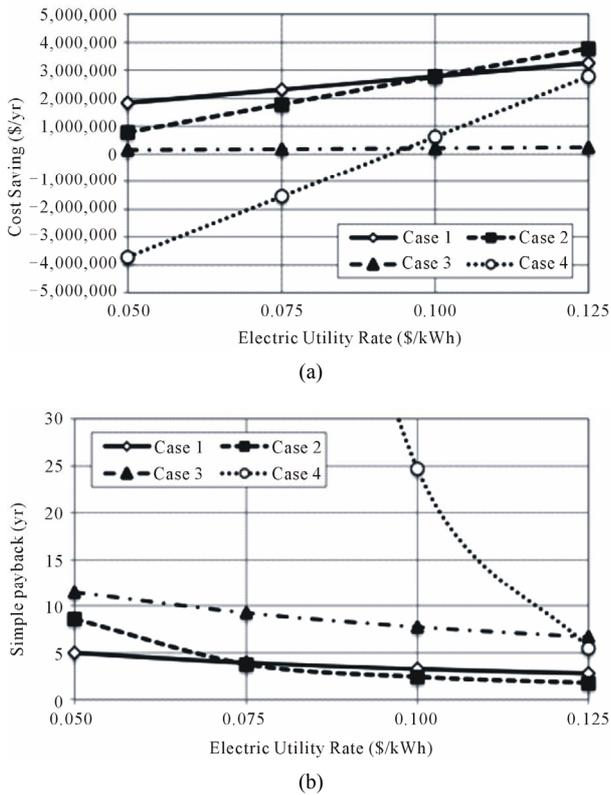
Figure 2. Effect of the electric utility rates on (a) the annual cost savings (b) the simple payback.
