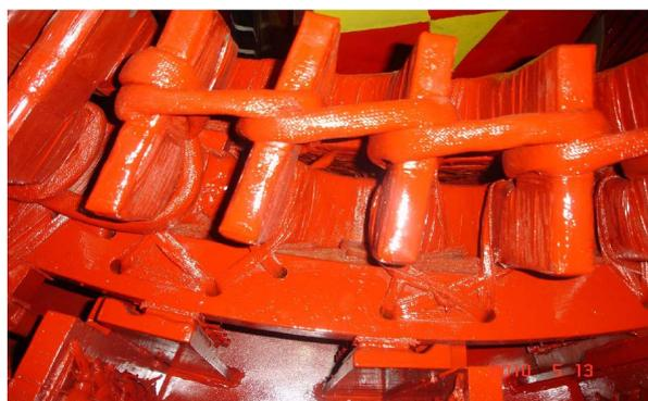
**Figure 7. Rectification measure: a continuous resin rope integrating bar-head joints.**
