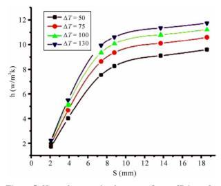
Figure 5. Natural convection heat transfer coefficients for different heat sinks.
