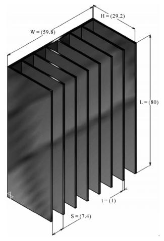
Figure 2. Fin configuration geometry.
