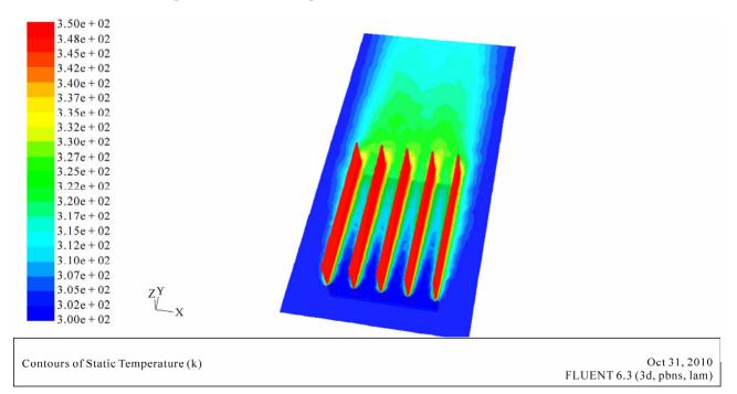
Figure 7. Variation of temperature contour of the heat sink (*s* = 13.7 mm).
