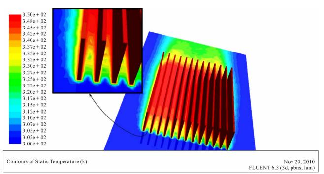
Figure 6. Variation of temperature contour of the heat sink (s = 3.9 mm).
