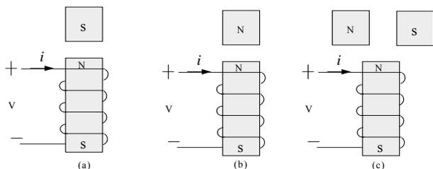
**Figure 2. Magnetic fields (a) saturated magnetic field, (b) linear (non-saturated) magnetic field and (c) middle case.**
