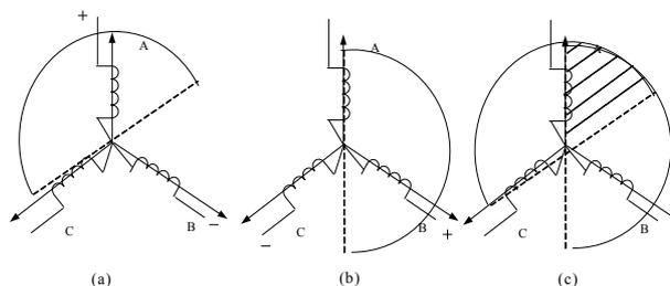
**Figure 3. The schematic diagram of initial rotor position detection. (a) Energized stator winding and rotor position within 180°; (b) Rotor position within 60°.**
