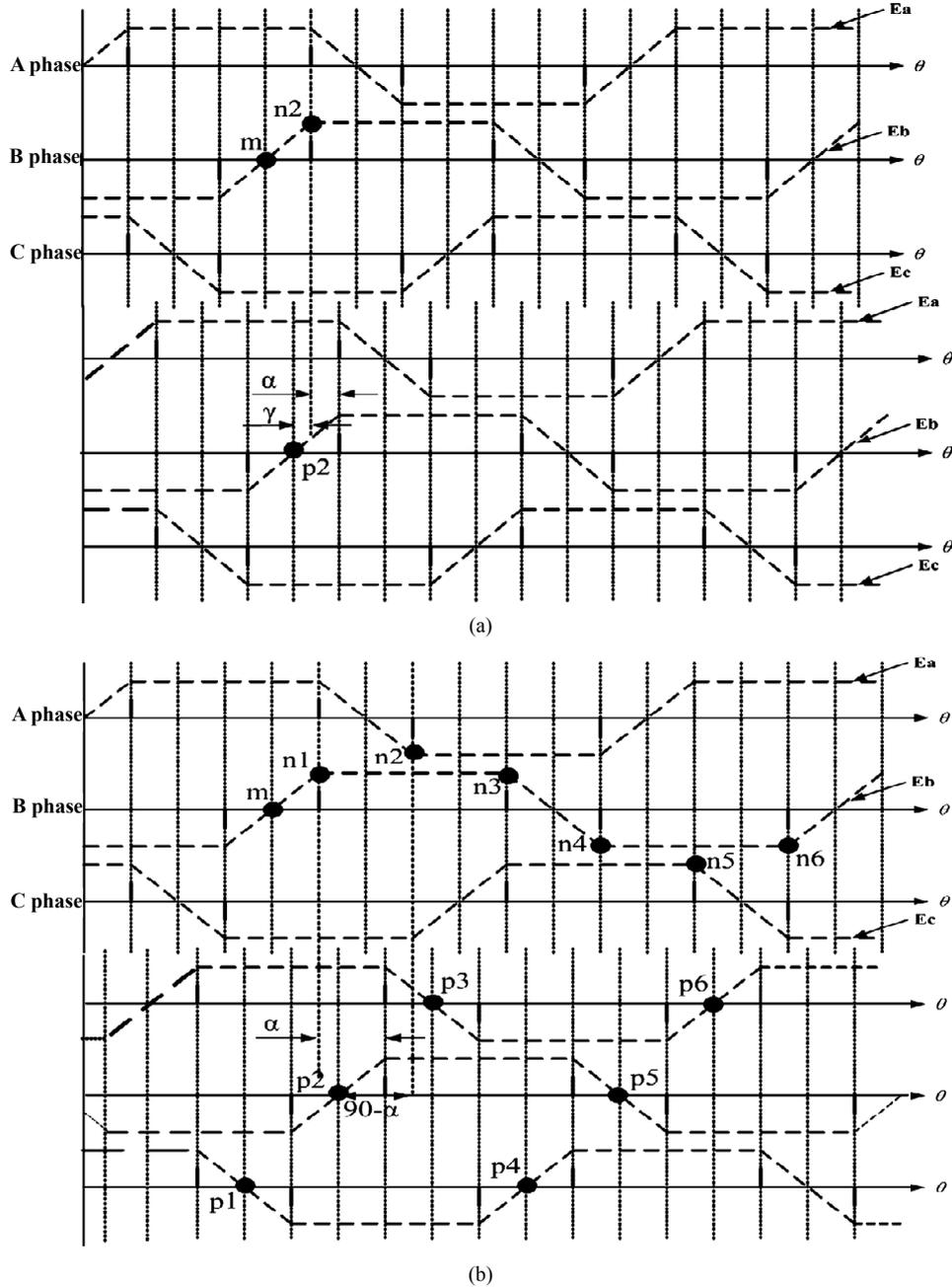
Figure 4. Lagging  $90^\circ - \alpha$  commutation method.
