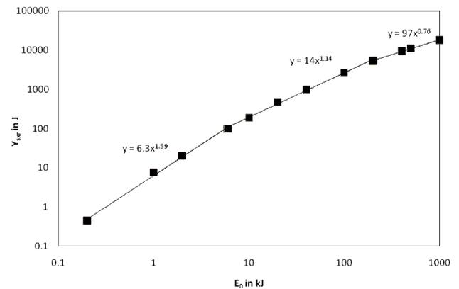
Figure 5.  $Y_{sxr}$  vs  $E_0$ . The parameters kept constants are:  $RESF=0.1$ ,  $c=1.5$ ,  $L_0=30$ nH and  $V_0=20$  kV and model parameters  $f_m, f_c, f_{mr}, f_{cr}$  at 0.06, 0.7, 0.16 and 0.7 respectively. The scaling deterioration observed in this Figure is discussed in the Conclusion section
