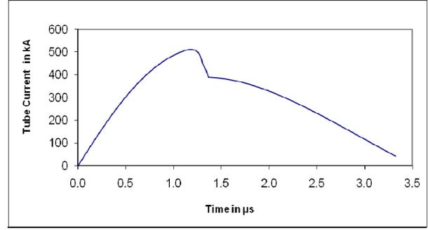
Figure 4. Computed total current versus time for  $L_0=30$  nH and  $V_0=20$  kV,  $C_0=30$  μF,  $RESF=0.1$ ,  $c=1.5$  and model parameters  $f_m, f_c, f_{mr}, f_{cr}$  are fixed at 0.06, 0.7, 0.16 and 0.7 for optimised  $a=2.285$ cm and  $z_0=5.2$ cm
