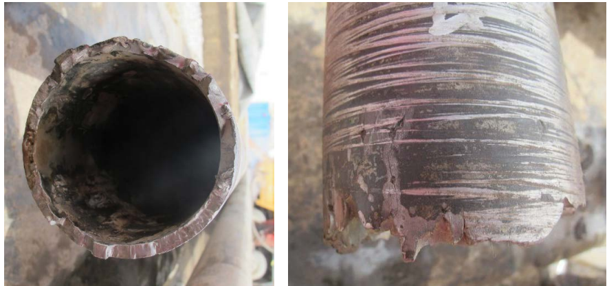
Figure 2. Morphology of root break of 418 tubing.
