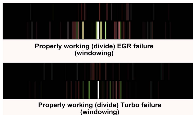
Figure 8. The result of the graphical divide function application between the layers, being the results of the wavelet analysis; black indicates the places that differ; original signals were subjected to windowing (Flattop).
