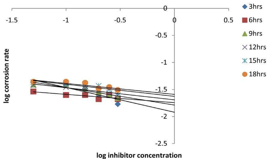
Figure 2. Variation of log corrosion rate log concentration of SDS for corrosion of copper in 2M HNO<sub>3</sub> at 30°C.
