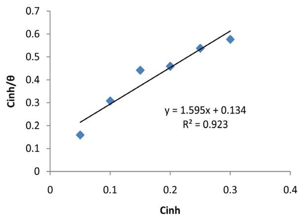
**Figure 3.** Langmuir adsorption isotherm for the corrosion inhibition of copper with SDS at 30°C.
