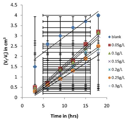
Figure 1. Volume of gas evolved versus time of copper in 2M HNO<sub>3</sub> with and without of SDS at 30°C.
