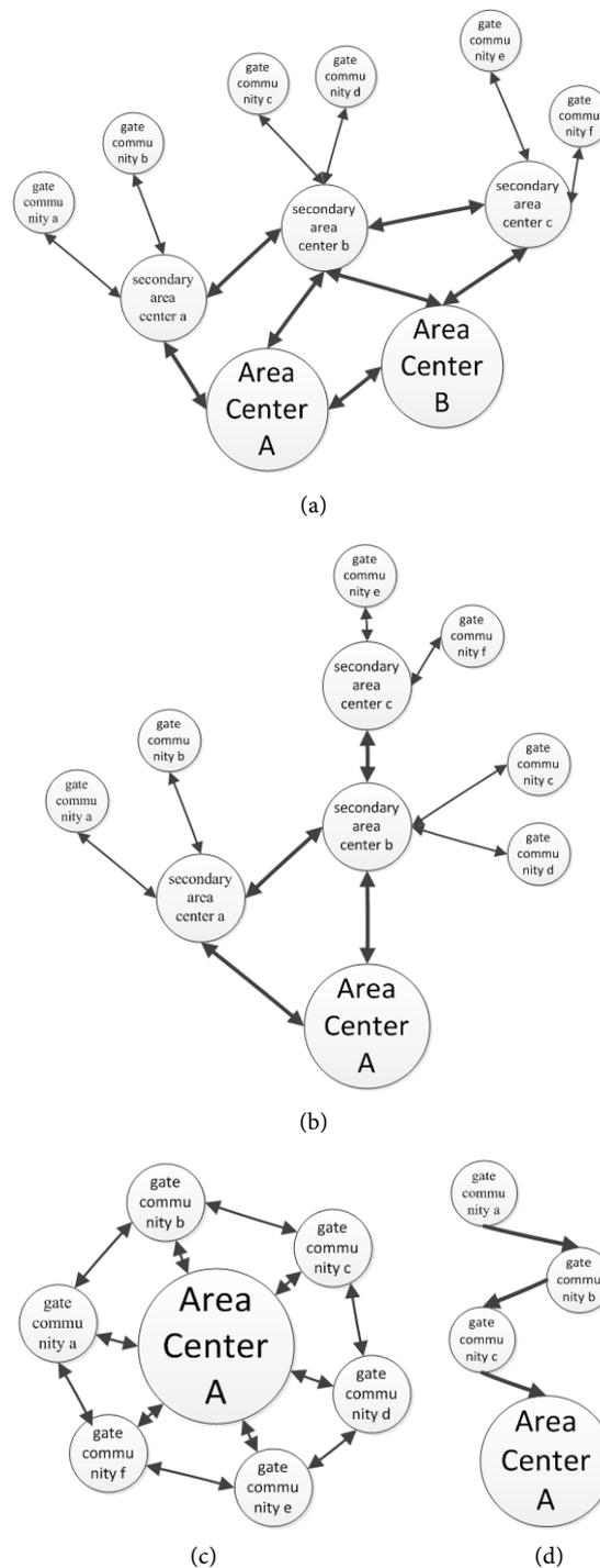
**Figure 3.** Visualization of boundary road structure and traffic flow. (a) Grid type; (b) tree type; (c) loop type; (d) linear type.
