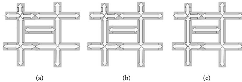
**Figure 2.** Three typical types of internal road structures in gated communities. (a) linear type; (b) grid type; (c) inter-loop.
