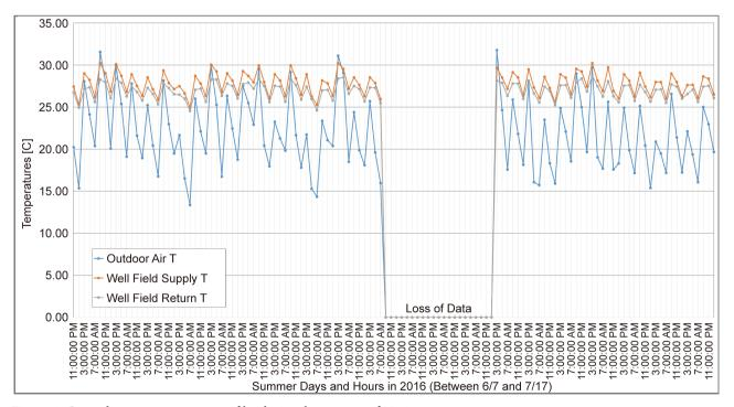
Figure 4. Ground water temperature profiles during the summer of 2016.
