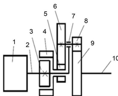
**Figure 1.** The scheme of the mechanism connection. (1. Synchronous motor. 2. Motor shaft. 3. Rotor of the excitation generator. 4. Stator of the excitation generator. 5. Central wheel. 6. Satellite. 7. Planet carrier of the differential. 8. Satellite. 9. The second central wheel. 10. Output shaft.)
