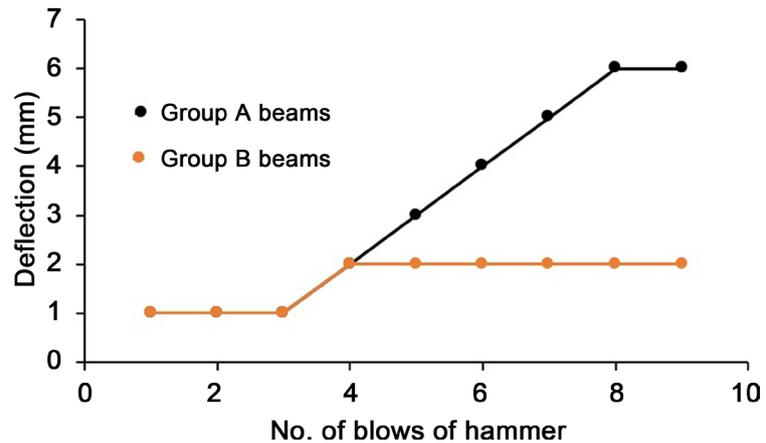
**Figure 5.** Impact load versus deflection response of RBC beams of group A (with two 12.7 mm diameter steel bars) and group B (with two 15.8 mm diameter steel bars).
