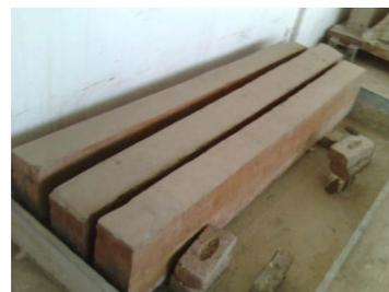
**Figure 2.** A view of baked clay beams.
