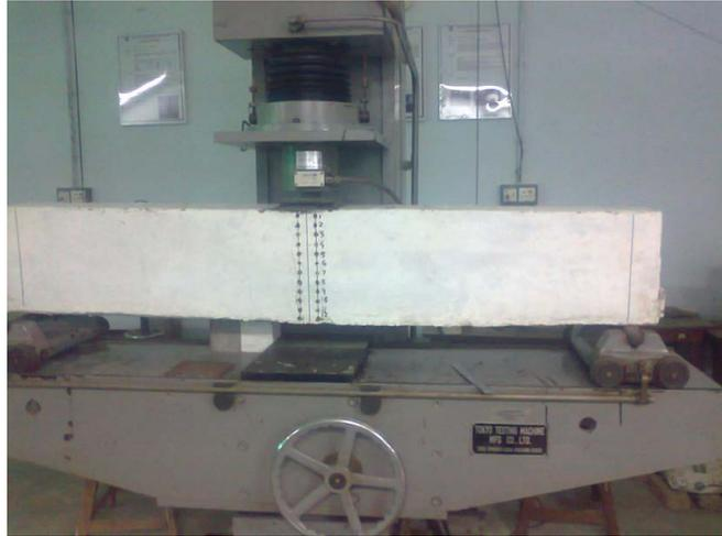
**Figure 4.** A reinforced baked clay beam is being tested in universal beam testing machine.
