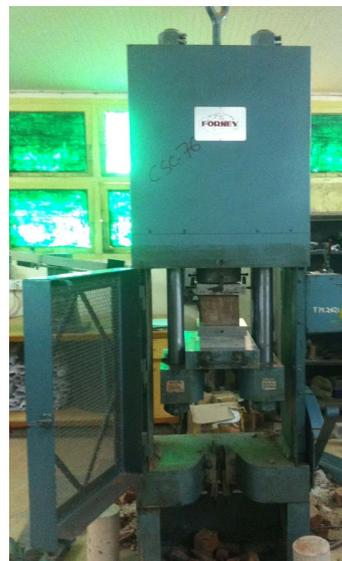
Figure 3. Baked clay cubes are being tested in universal testing machine.
