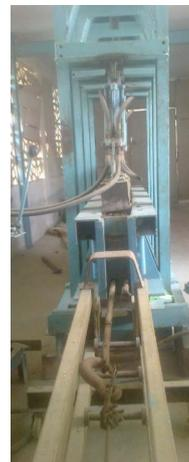
**Figure 1.** Mechanized system for casting and pressing of clay beams [12].
