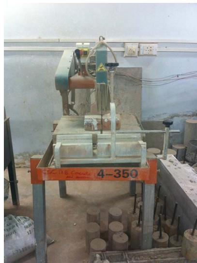
**Figure 6.** A baked clay brick is being cut into two halves using cutter machine.
