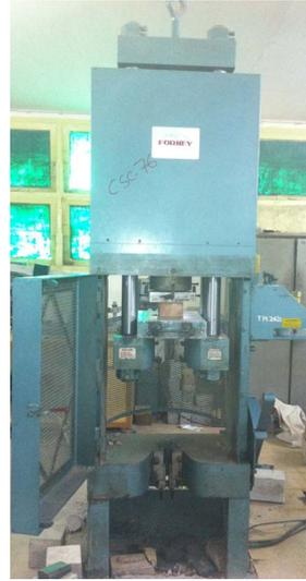
**Figure 7.** A baked clay brick specimen is being tested for compressive strength in Universal Testing Machine.
