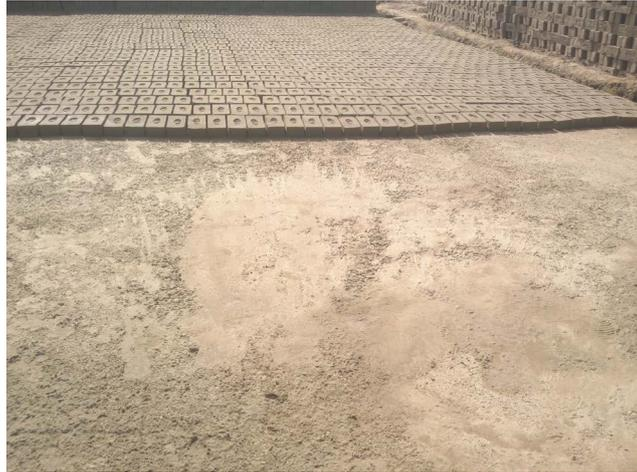
**Figure 4.** Clay bricks are being placed on ground for drying.
