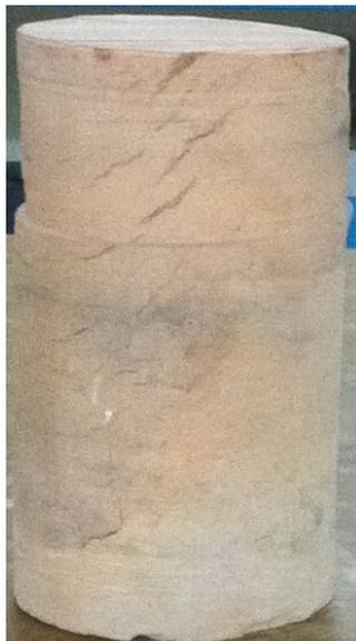
**Figure 3.** A baked clay cylinder core of 150 mm diameter and 300 mm height.
