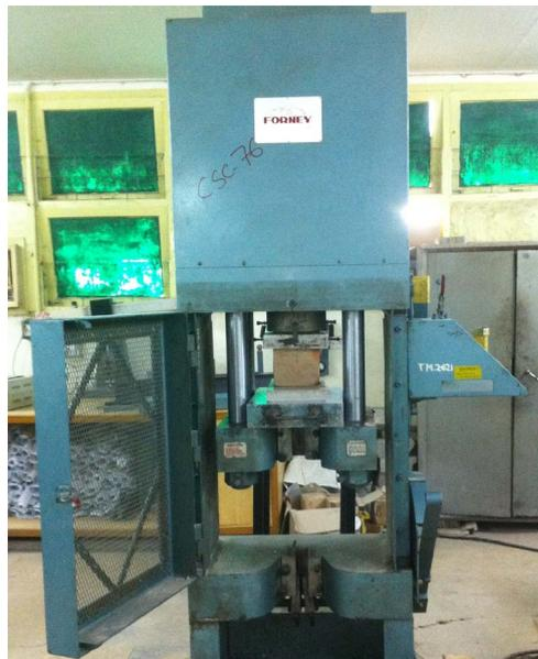
**Figure 4.** Baked clay cubes of 150 mm size are being tested in Universal Testing Machine.
