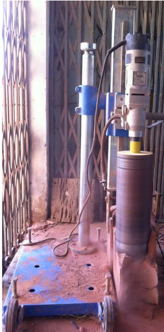
**Figure 2.** A baked clay cylinder is being cut with core cutter machine.
