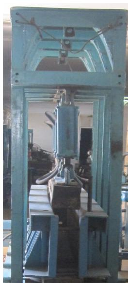
**Figure 1.** A clay beam is being cast and compacted in a Mechanized System.
