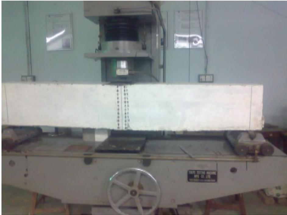
**Figure 6.** A white washed reinforced baked clay beam is being tested using Torssee's beam testing machine.
