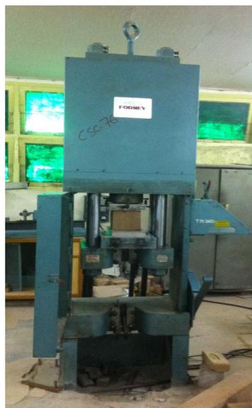
Figure 5. Baked clay cubes of 150 mm size are being tested in Universal Testing Machine.
