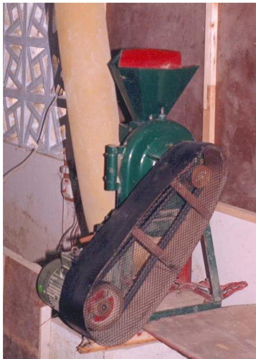
Figure 1. Clay, obtained from the quarry containing lumps, is ground in Pulverizer.
