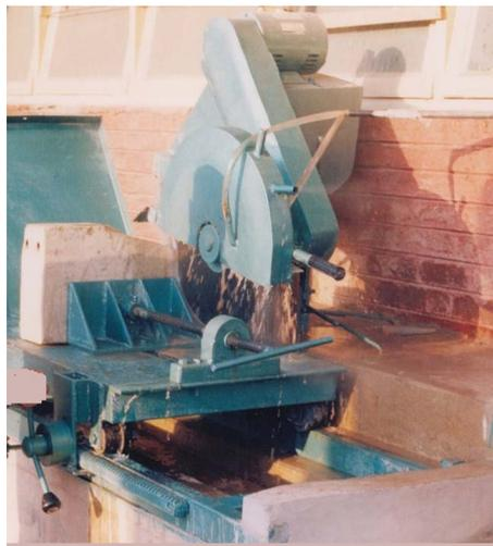
Figure 4. Baked clay cubes of 150 mm size are sawed using cutter machine.
