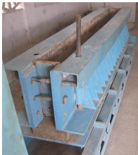
Figure 1. Mould utilized for casting of clay beams.
