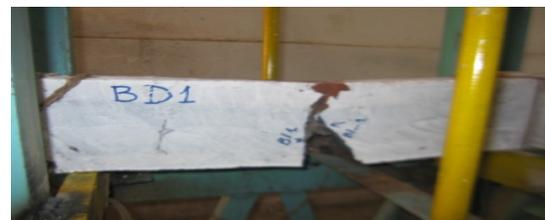
Figure 6. Failure behaviour of reinforced baked clay beam of grade 30 under impact load.
