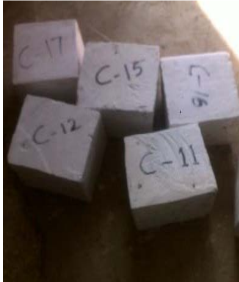
Figure 4. 150 mm size cubes sawed from baked clay beams.
