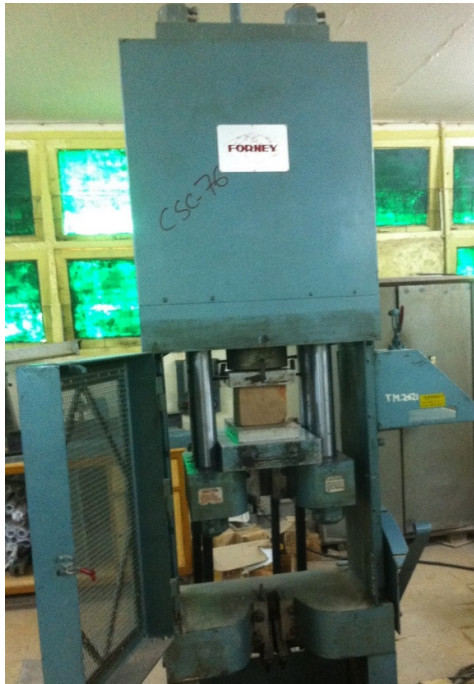
Figure 5. Baked clay beams being tested in universal testing machine.
