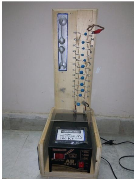
**Figure 1.** High voltage lightning impulse generator.
