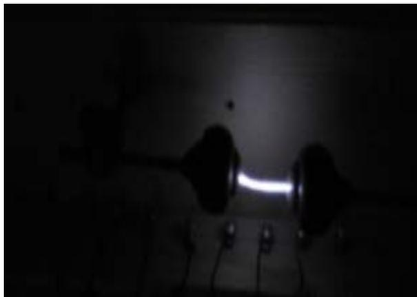
**Figure 4.** 100 kV lightning spark.
