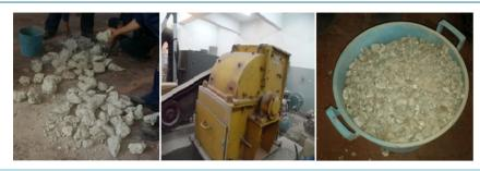
Figure 2. Different phases for preparing recycled, crushing and sieved CDW.
