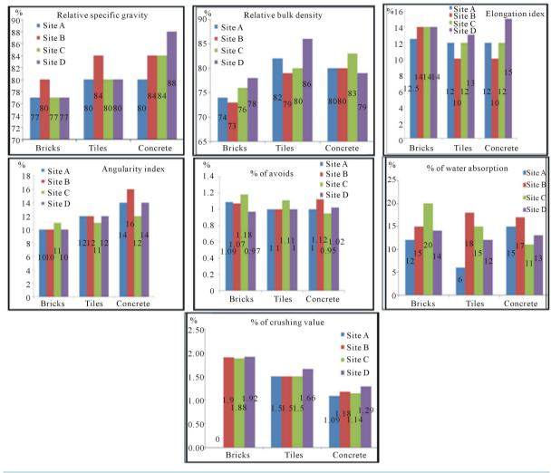
Figure 4. Shows the relative properties of all types of the recycled aggregate.
