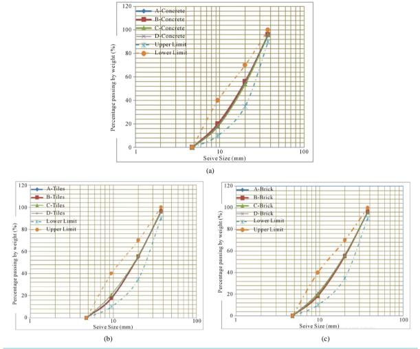
Figure 3. Grading curves for recycled aggregate with respect ECP limits. (a) Concrete in all sites; (b) Cement tiles in all sites; (c) Red brick in all sites.
