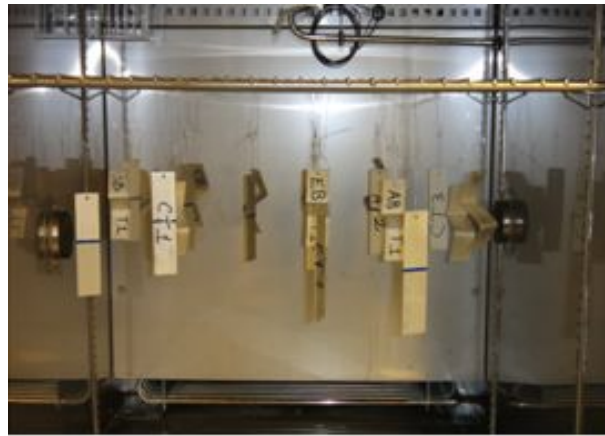
Figure 1. Coupon arrangement in the thermotron environmental test chamber for hydrothermal exposure.
