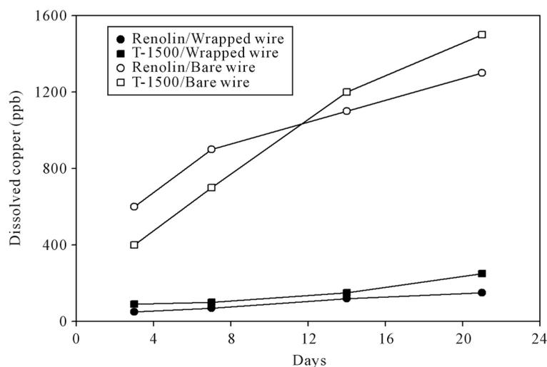
**Figure 3.** Barrier properties of the paper layer: the copper release kinetics from bare and paper-wrapped copper wire are compared. Sealed-tube experiment at 150°C. The characteristic copper fluxes are ca  $1 \times 10^{-8} \text{ g}\cdot\text{m}^{-2}\cdot\text{s}^{-1}$  for the paper-wrapped wire and ca  $1.0 \times 10^{-9} \text{ g}\cdot\text{m}^{-2}\cdot\text{s}^{-1}$  for the bare wire.
