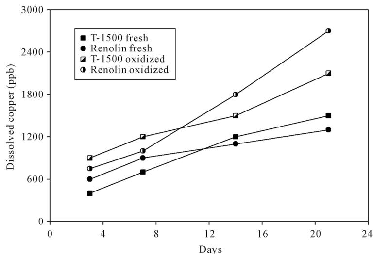
**Figure 4.** Effect of paper degradation products on oil corrosiveness towards copper (sealed-tube experiment with bare copper wire, 150°C).
