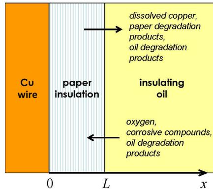
**Figure 6.** Mass transport processes occurring in the paper-oil insulation system during the ageing process.
