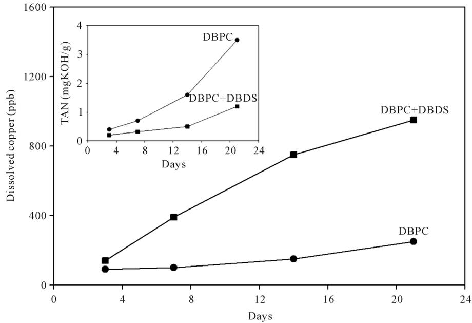
**Figure 5.** Effect of DBDS on copper release and oil oxidation kinetics. (Open-tube experiments with a DBPC-inhibited commercial product T-1500 and paper-wrapped copper wire at 150°C, the concentration of DBDS was 500 ppm).
