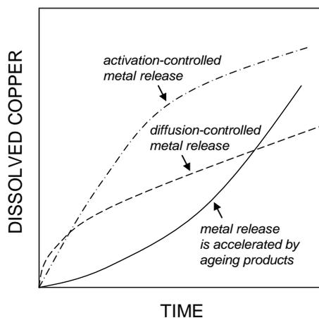
**Figure 7.** Characteristic copper release curves for various kinetic scenarios.
