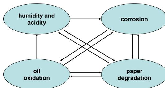
**Figure 1.** Interaction between different degradative processes occurring in oil-immersed transformers.
