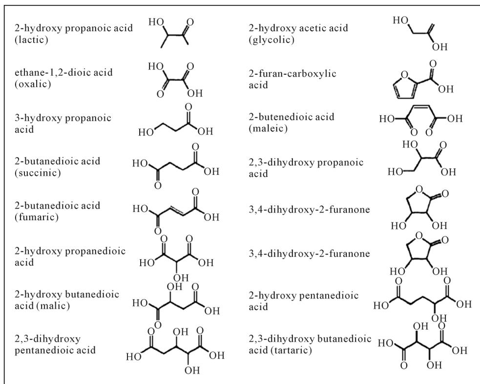
**Figure 2.** Carboxylic acids produced as a result of oxidative degradation of paper [27].
