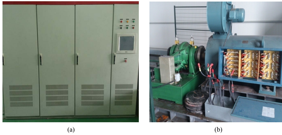
Figure 7. Experimental platform of nine-phase induction motor propulsion system. (a) 9-phase inverter; (b) 9-phase induction motor and power testing machine.
