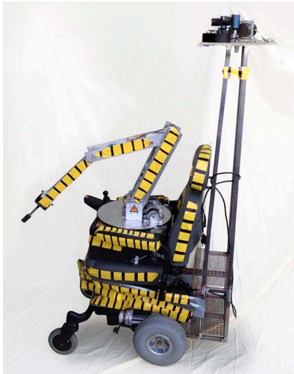
Figure 4. A photograph of the RRC-controlled motorized power wheelchair. A 4-degree of freedom robotic arm, mounted on the wheelchair, is shown in the photograph. The tactile system is represented by pressure transducers taped onto the wheelchair, with one pressure transducer located under each patch of tape. The visual system, presented in greater detail in Figure 7 , is also shown mounted on the wheel chair.
