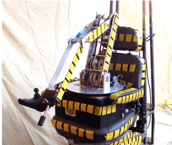
Figure 6. A close up view of the robotic arm used to behaviorally program proprioceptive knowledge into the system.
