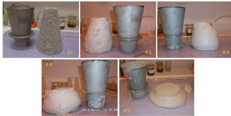
Figure 4. Slumping behaviors of concrete.
