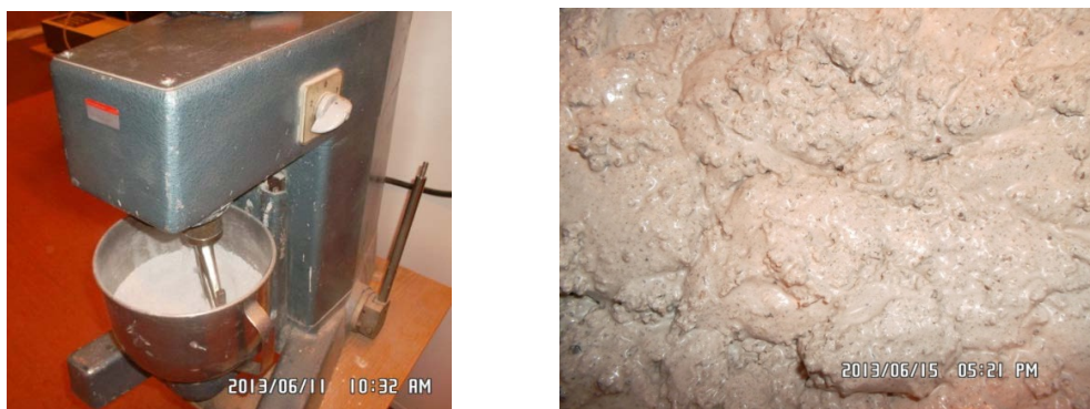
Figure 2. Concrete mixture preparation with the degree of fluidity being illustrated by the right photo.
