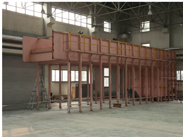
Figure 7. Full-width weir for Cheongpyeong Dam test.
