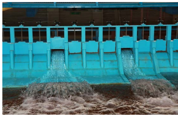
Figure 15. Impact of sluice gate interference (case 4).
