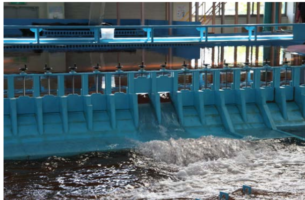
Figure 14. Impact of sluice gate interference (case 1).
