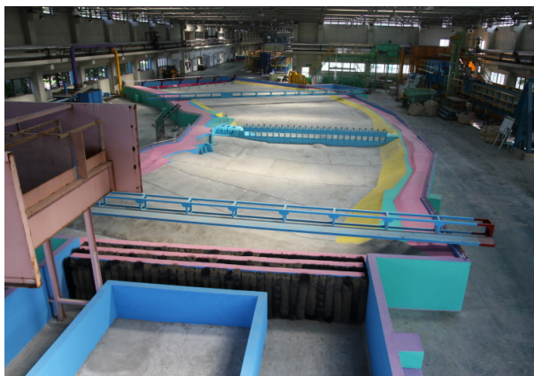
Figure 6. Cheongpyeong Dam hydraulic model.
