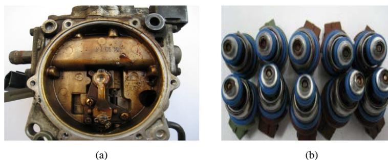
**Figure 1.** The contamination in vaporizer and injector from LPG vehicles. (a) Vaporizer contamination; (b) Injector contamination.
