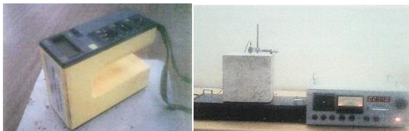
Figure 2. Moisture meter (left), cube placed on dynamic modulus meter (right).
