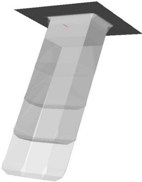
Figure 3. Etching profile evolution during equidistant time steps (0 s, 30 s, 60 s, 90 s and 120 s).
