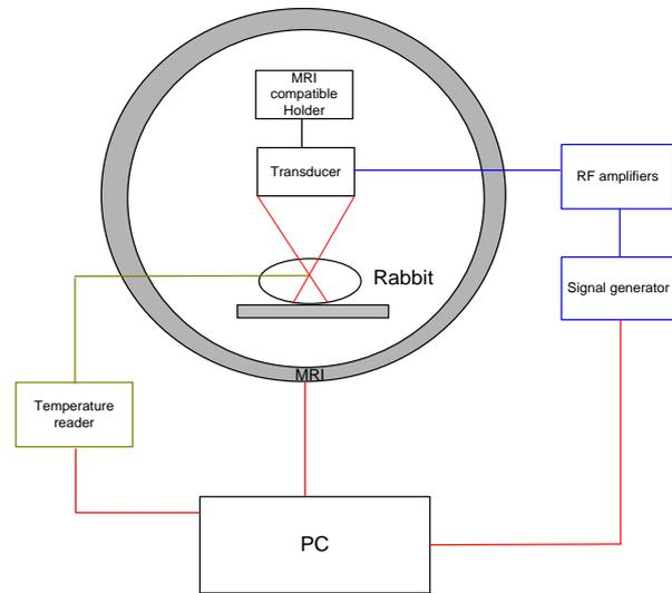
**Figure 1.** MRgFUS system for *in vitro* sonothrombolysis.
