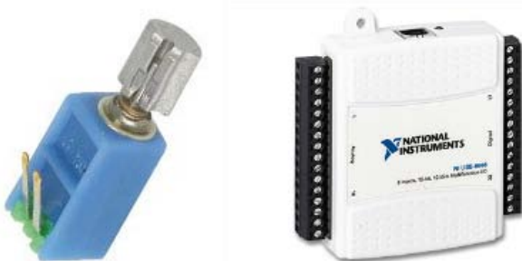
Figure 2. Left vibration motor and right NI-USB card.
