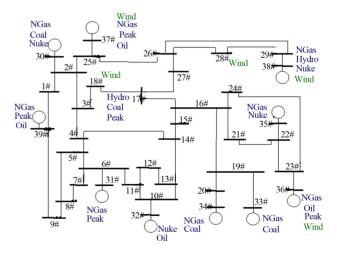
Figure 7. 39 Bus power system test system.
