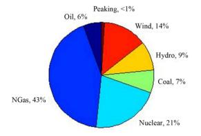
Figure 9. Generator dispatch by fuel type—10% wind penetration.
