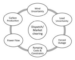
Figure 1. Sub-models within the Monte Carlo-Optimal Power Flow modeling framework.
