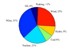
Figure 10. Generator dispatch by fuel type—20% wind penetration.
