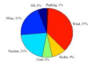
Figure 11. Generator dispatch by fuel type—30% wind penetration.
