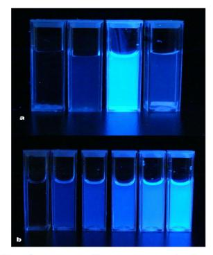
Figure 5. a(top, l. to r.) Fluorescent response of untreated cotton nanocrystals, tetrapeptide-nanocellulose, tetrapeptide-nanocellulose with 2 U/mL of HNE and tetrapeptide-filter paper with 2 U/mL of HNE. b(bottom) fluorescent response of the tetrapeptide in solution at different concentrations ranging (l. to r.) 0 to 0.25  $\mu$ mole/mL with 2 U/mL of HNE.
