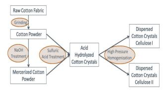
Figure 2. Schematic flowchart of the preparation of cotton cellulose nanocrystals.
