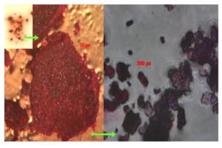
Figure 6. Cellulose nanocrystals after released pNA has reacted with the color amplifying reagent.
