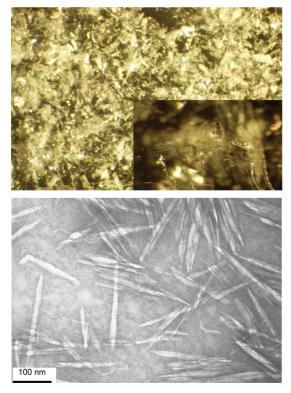
Figure 1. a(top) Untreated freeze-dried cotton nanowhiskers magnified 15X and 60X(inset). b(bottom) TEM of cotton nanowhiskers.
