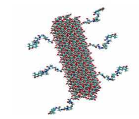
Figure 4. Model of peptide-conjugated cellulose nanocrystal. Six tetrapeptides (Succinyl-Ala-Ala-Pro-Val-CMA) with amino-terminal of peptide attached to glycine-cellulose (see Figure 3).
