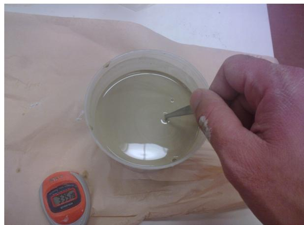
**Figure 6. Preparation of grout. Notice the fluidity.**
