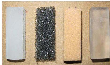
**Figure 4.** A picture of objects used for grasping: (from left to right) PVC ( $O_1$ ), Foam ( $O_2$ ), Ethaflex ( $O_3$ ) and Plexiglass ( $O_4$ )
