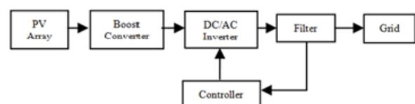
**Figure 1.** Basic concept of grid connected inverter.
