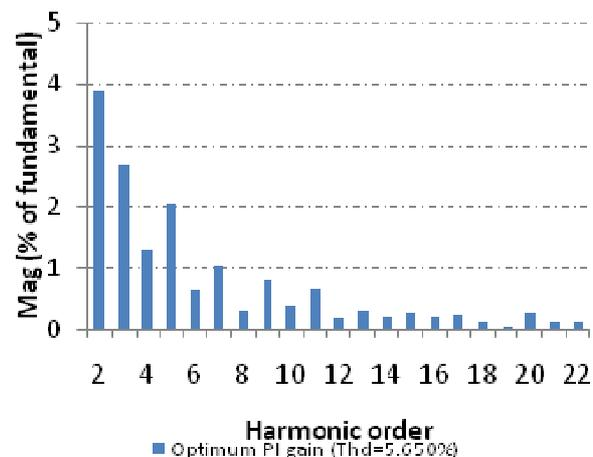
**Figure 7.** Harmonic spectrum of PI current controller.
