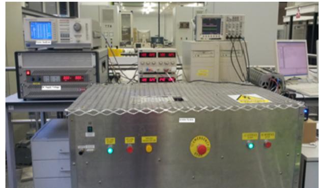
**Figure 6.** Experimental test setup for inverter system.
