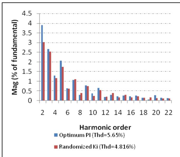
**Figure 10.** Harmonic spectrum comparison.
