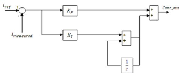
**Figure 4.** Block diagram of PI current controller.
